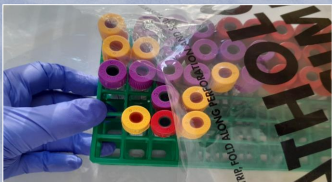
3 – Place the rack inside the singular plastic bag, with absorbent pad
